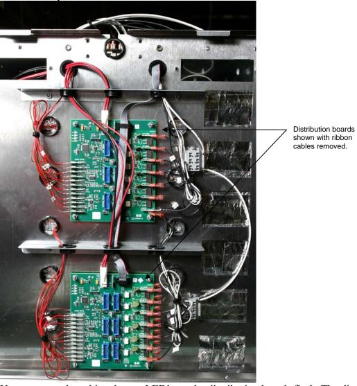
Upon startup, the cabinet beeps. LED's on the distribution boards flash. The displays show the version number of the cabinet's firmware and then the row's status.
